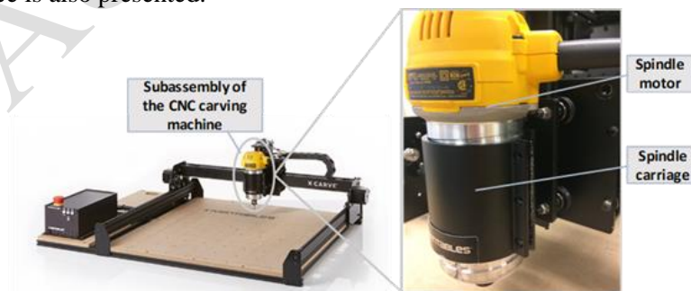
Figure 13: The spindle subassembly of a CNC carving machine.
