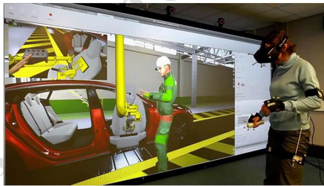
Figure 11: A operator wearing an Oculus headset for immersive VR and attached with multiple markers for motion tracking (Image courtesy of OPTIS) [11].
